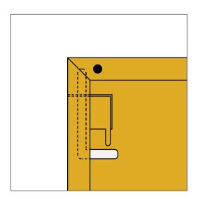
At the top of the door, insert the L shape post up into position through the holes.
